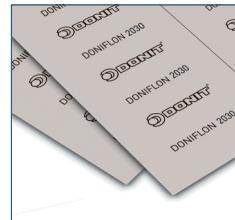
DONIFLON® 2030 is structurally enhanced PTFE gasket sheet filled with barium sulfate. It has outstanding chemical resistance to various media, same as DONIFLON® 900E; especially recommended for strong alkaline solutions under moderate temperatures and hydrofluoric acid (up to 48%). This material has enhanced creep performance compared to plain PTFE material. It is the ideal gasket material for equipment where higher bolt loads are required.
