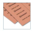
DONIFLON® 2020 is structurally enhanced PTFE gasket sheet filled with silica. It has outstanding chemical resistance to various media, same as DONIFLON® 900E; especially recommended for inorganic acids in all concentrations, except hydrofluoric acid. This material has enhanced creep performance compared to plain PTFE material. It is recommended for pharmaceutical and food industries as well as LNG & cryogenic applications.
