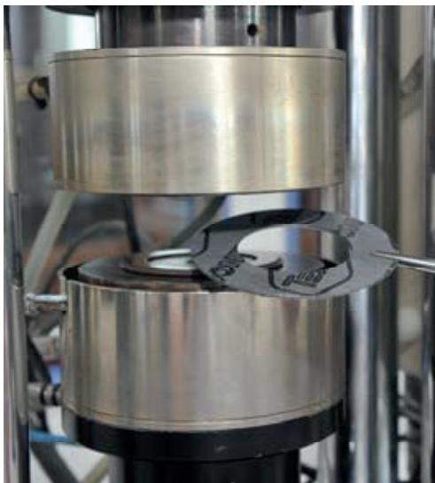
Figure 5: Test rig for hot compression test
