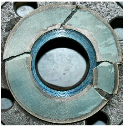
Figure 1: Damaged gasket without anti-stick coating
